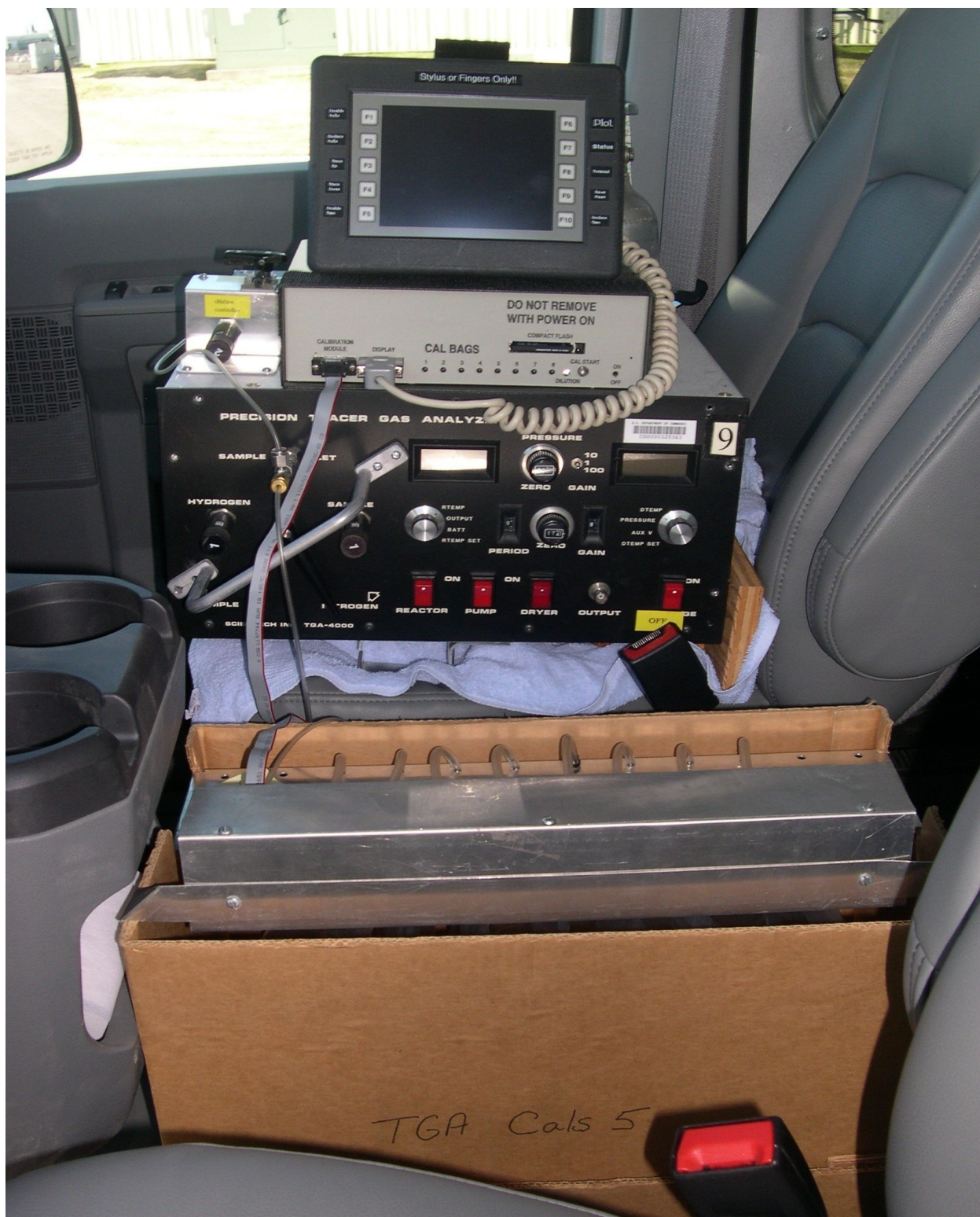
Figure 46. NOAA mobile, fast response, tracer gas analyzer installed in the passenger seat of a van. A calibration box is visible in the foreground. The microcontroller that collects the data and runs automated calibrations is attached to the top of the instrument.
