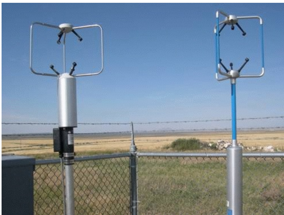
Figure 51. A closeup picture of an R. M. Young Ultrasonic 81000 (left) and a Gill Windmaster Pro (right) used during PSB2.
