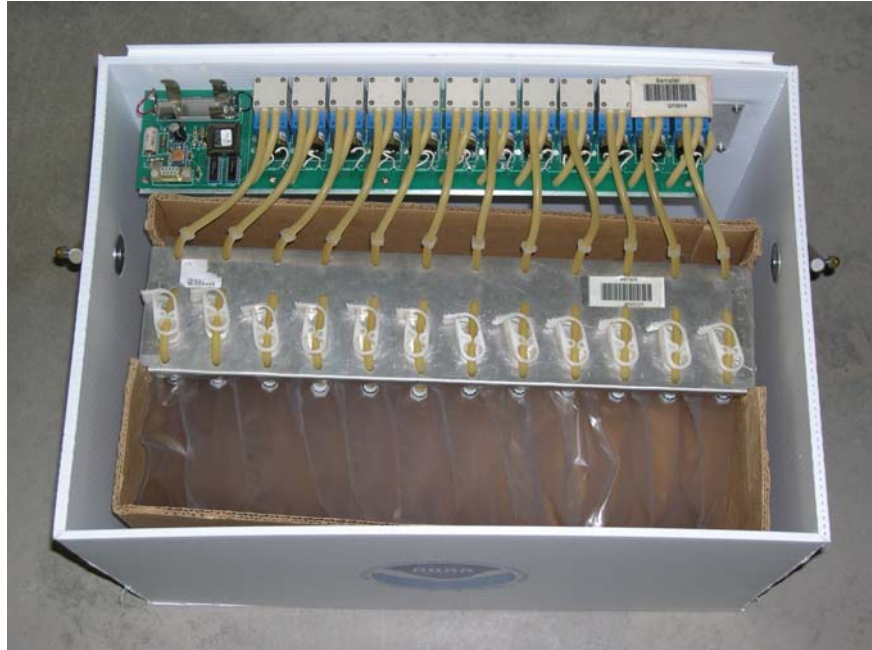
Figure 19. Bag sampler with sampler cartridge installed.
