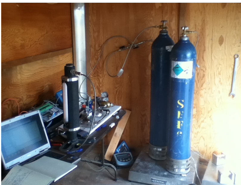
Figure 7. The SF 6 release system inside the cargo trailer including the SF 6 bottles, mass flow controller, computer data acquisition and control system, and electronic scales under the bottles.
